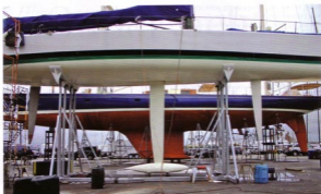
A handicapper's nightmare, different hull configurations with low wetted surface (Morning Glory) and moderate wetted surface (Rebecca) behind. Morning Glory is extremely fast in light winds, while Rebecca is much more comfortable.
